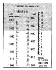
Values can be read directly from the scales. The sharp definition of contrast between the light and dark fields seen through the eyepiece assists accurate readings.
